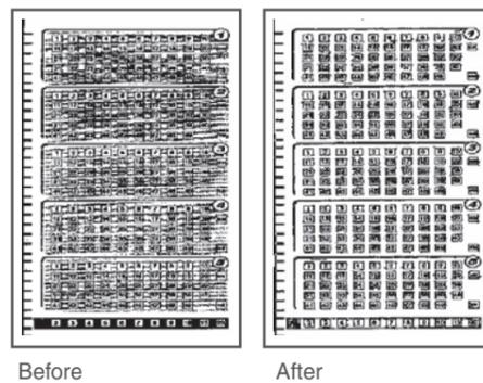
The SmartThreshold function enables Microtek's scanners to define the best level of a threshold used in high-contrast and black-and-white images automatically, improving the clearance and readability of black-and-white documents.
