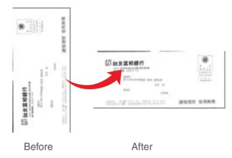
The Auto Document Rotation function enables the scanner to rotate each saved image into a readable direction automatically based on specified OCR language. Users do not need to rotate the document manually when scanning, saving time and energy.
